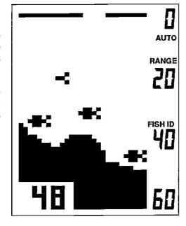
MODE 2 - This is the same as mode 1 except it has FASTRAK. This displays on the right side of the screen. It converts all echoes to horizontal bars when they first appear on the screen. This gives a rapid update of conditions directly under the boat. Echoes are also scrolled normally across the display. The Fish I.D. feature is not available with this mode.
